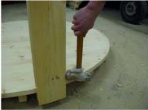
Put a pencil mark on the first stave that you fix to the base. Position the first stave, so that it covers one of the two longest floorboards.
